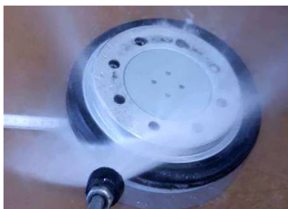
High pressure Water spray test 100 bar (1.45 ksi)
